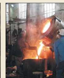
Pouring the molten metal into a ladle.
