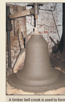
A timber bell crook is used to form the shape of the bell.
