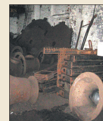
Bell moulds in the Casting Hall.
