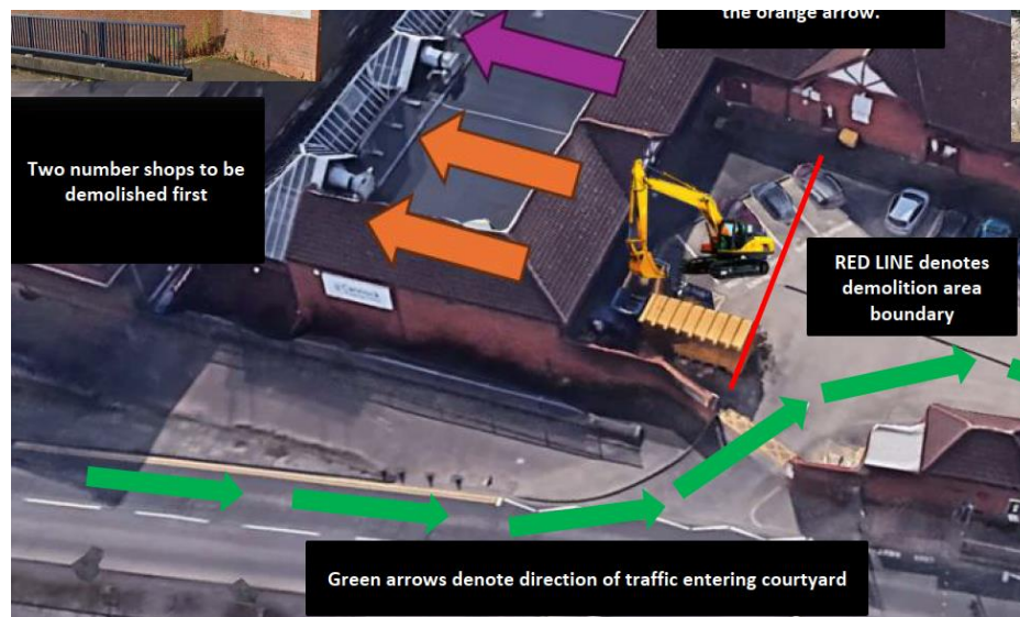
Figure 3: Extract from Demolition Method Statement. Demolition of Units 1-3 will progress from the rear service yard following soft strip of materials
