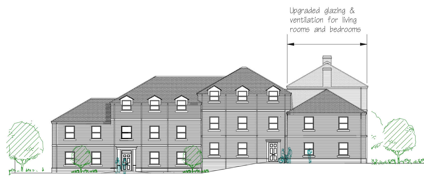
SIDE ELEVATION VIEW B
