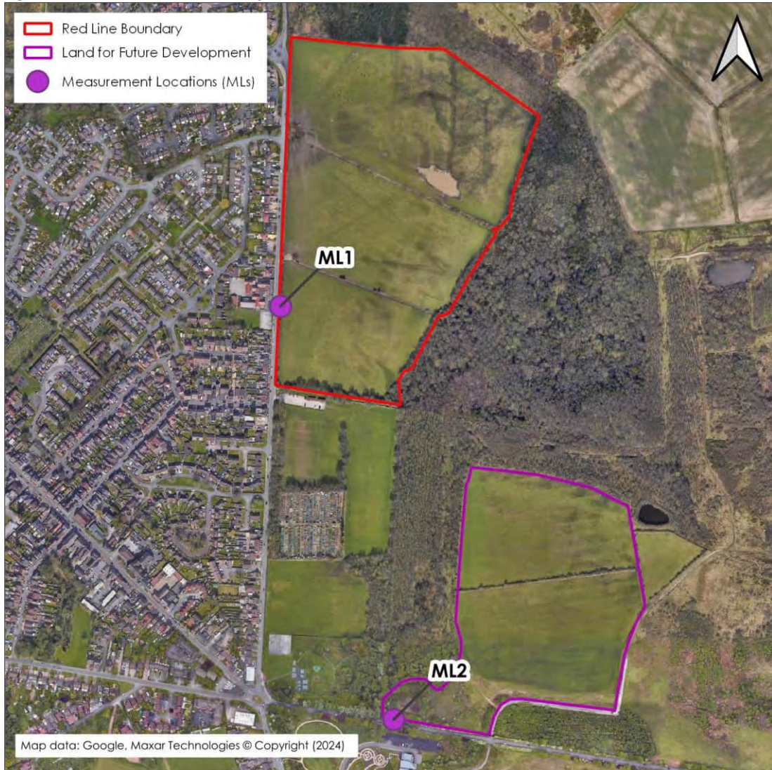
Figure 3.1: Baseline Noise Survey Measurement Location
