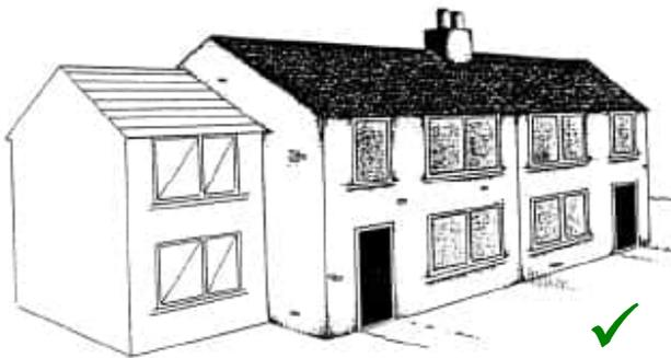
An extension is best designed to be subordinate to the existing building, i.e. not extending the full depth of the dwelling and should be set back from the front wall of the dwelling in recognition of its subordinate nature. Permitted development rights for ground floor extensions (up to 50% of the existing dwelling width) allow
